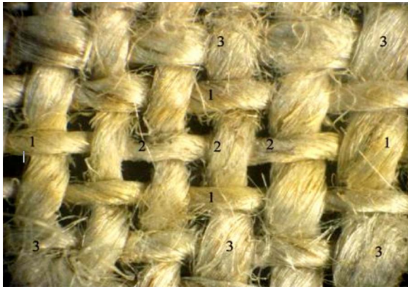
Figure 5. Linen area irradiated by ArF laser pulses having different characteristics corresponding to the local laser intensity value I(x, y) . (1) Colored area. (2) Ablated area where fibers are first colored and then vaporized. (3) Area irradiated below threshold for coloration.
